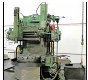
BULLARD CUT MASTER 42" VERTICAL TURRET LATHE
